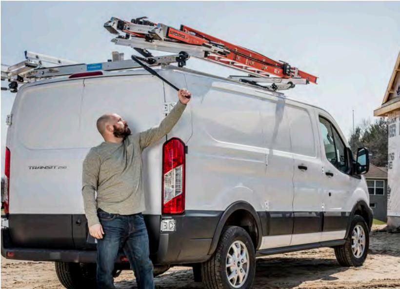
The new, simpler design makes it easier to install and adjust. The aluminum build of the rack reduces corrosion and keeps your ladder rack looking like new. It will accommodate a variety of ladders and safely secure them for transport.
